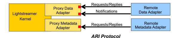
The Proxy Data Adapter and the Proxy Metadata Adapter are ready-made Adapters, written in Java and provided as part of the Lightstreamer Server. They expose the Data Provider and Metadata Provider interfaces over TCP/IP sockets.
